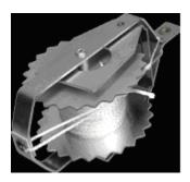
Twenty minutes before the schedule flight, the water-activated battery is soaked in water for at least 2-5 minutes.
